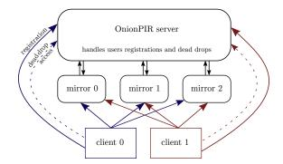
**Figure 3.1:** OnionPIR system model. Each client performs PIR queries via the mirror servers. The OnionPIR server handles user registrations, holds the database for the dead drops and distributes the PIR database to the mirrors. Client may connect to the OnionPIR server directly or via Tor.
