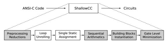
Figure 2.4: ShallowCC's compilation chain from ANSI-C to Boolean circuits [BHWK16]
