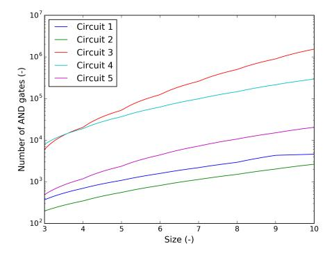
**Figure 6.1:** The number of AND gates in the different circuits for varying number of participants and topics in the assignment problem
