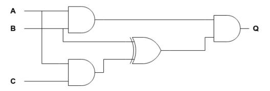
Figure 2.1: A Boolean Circuit with 3 inputs, 4 gates and 1 output
